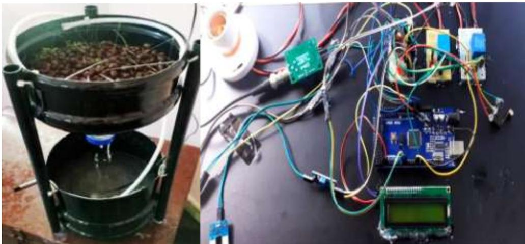
Fig.3 Hydroponic Gardening setup Fig.4 Hardware Circuit setup
